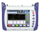
Employing superior micro-optic design and MEMS tuning technology, RXT and UX400 OSA test modules measure key optical parameters such as wavelength, channel power, and OSNR in CWDM and DWDM networks.
