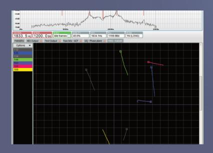
Krypto500 is for Narrowband (NB) signals up to 48 kHz in bandwidth principally found in HF. It enables even inexperienced signals analysts to quickly and accurately interpret information about a signal of interest.
