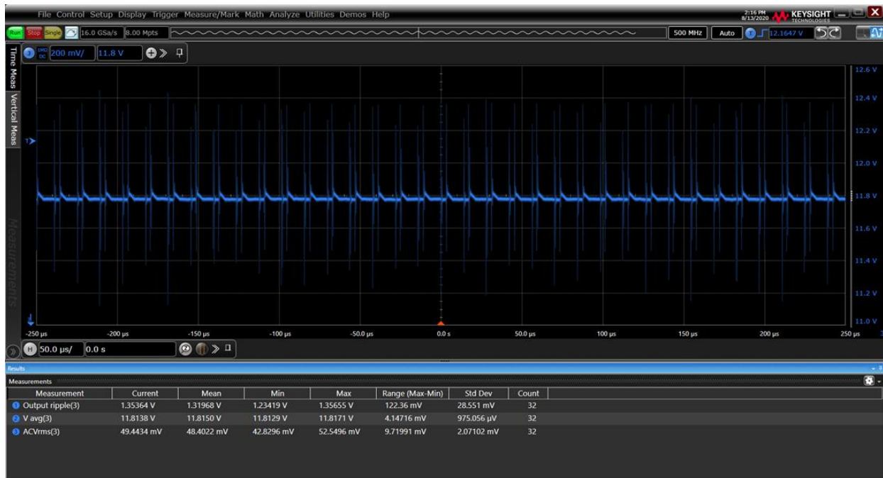
Figure 14. Output ripple measurements
