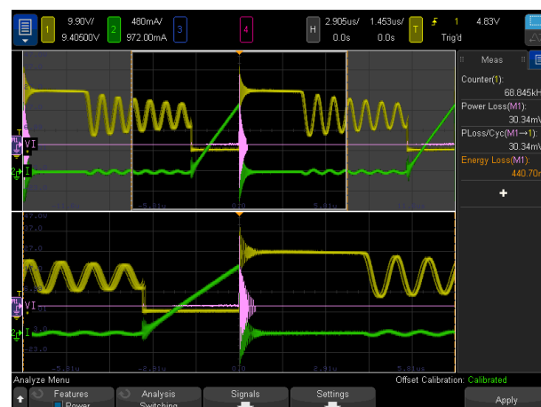
Figure 5: Switching loss measurement using the MSOX4154AUT power “best” bundle.
