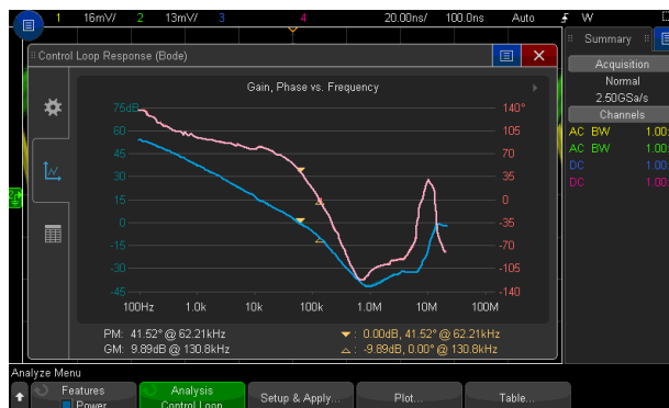
Figure 4: Control loop response test using the DSOX3054AUT automotive “better” bundle.
