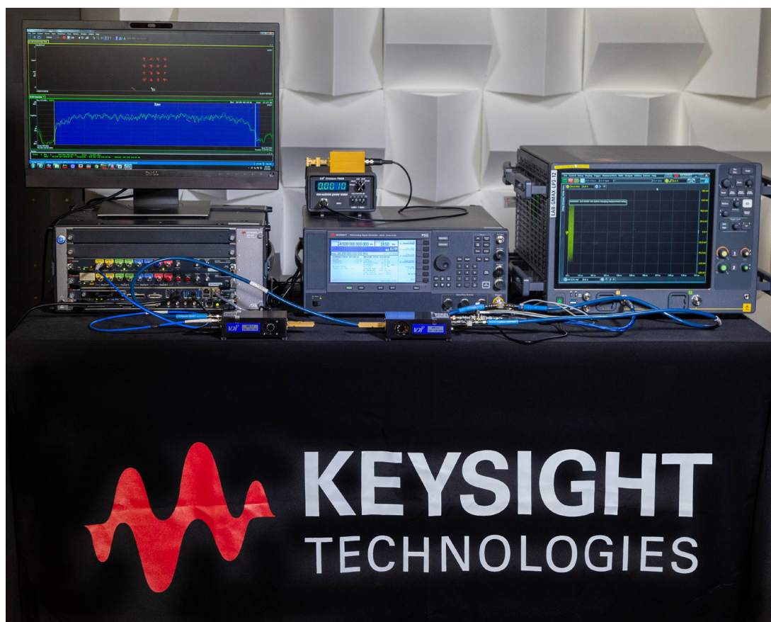
Figure 2. Sub-THz Testbed for H-Band, 220-330 GHz
